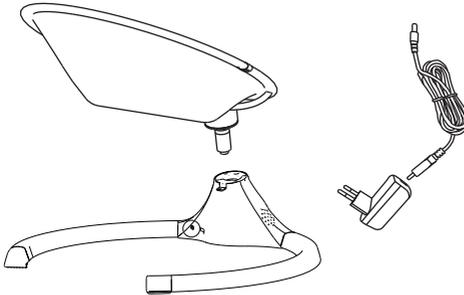
Plug the Power Adapter (D) into the DC jack located on the Base Frame (B).
